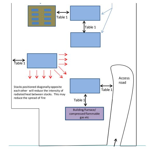
Figure 1: example of good pile layout
